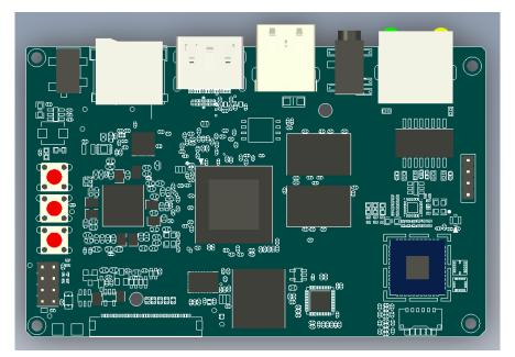
With a dimension of 101.9mm\*64.5mm\*1.6mm, JaguarBoard uses the high-performance CPU of Intel Atom Z3735G 4 and integrates a variety of interfaces. JaguarBoard allows more options for operating systems. In the same way as installing Ubuntu or Windows on PCs with a USB flash drive, you can install Ubuntu-14.10-desktop-amd64 or Windows 8.1or any other
